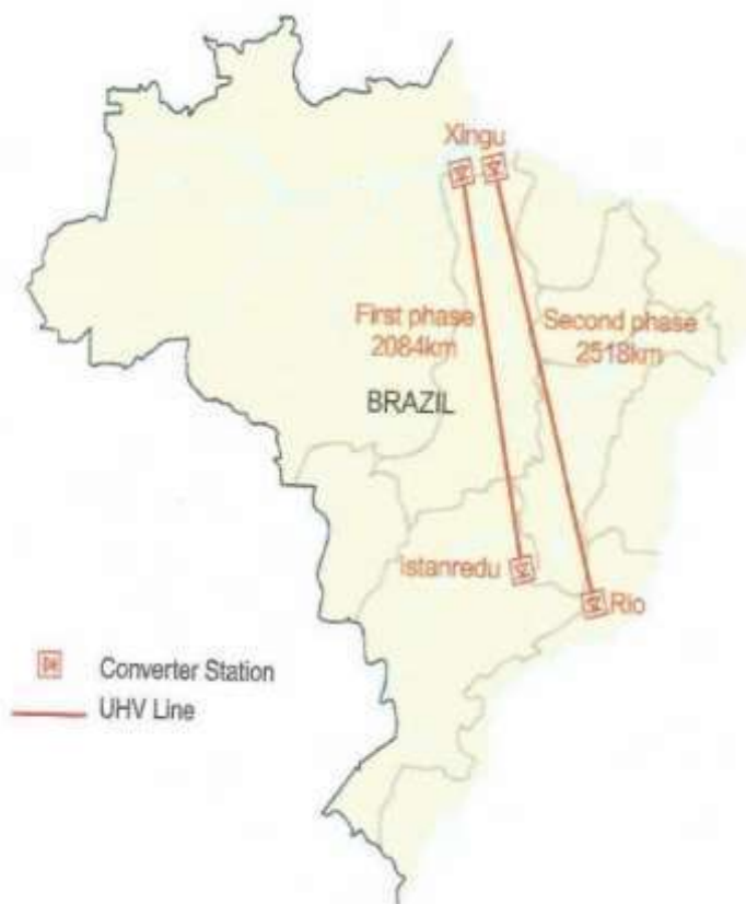
Fig. 2 - Belo Monte \pm 800 kV UHVDC Transmission Project [5].
