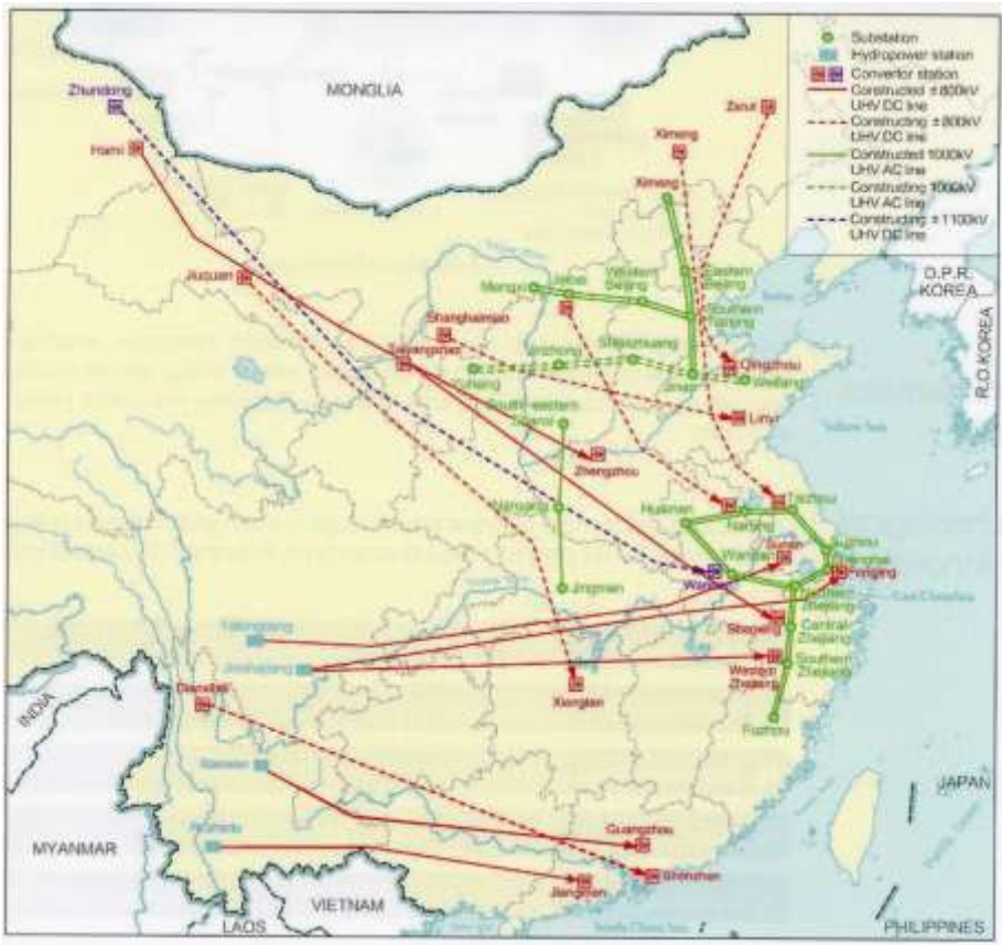
Fig. 1 - UHV grid projects in China [4].
